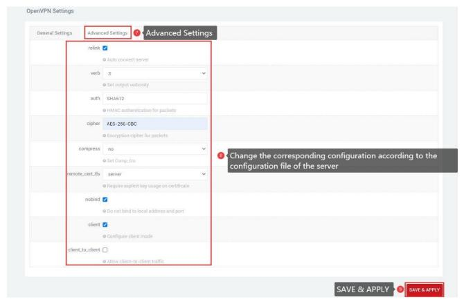
After the connection is successful, the status bar will refresh the address. If openvpn is not used, uncheck it and click "SAVE & APPLY".
