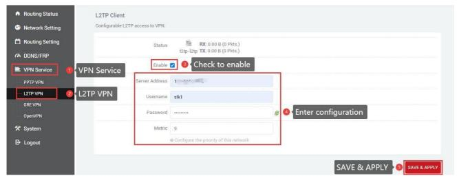
After the connection is successful, the address assigned by the server will appear in the status bar. If I2tp is not used, uncheck it and click "SAVE & APPLY".
