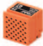
#29, #30, #35 Temperature, humidity, and pressure meters
