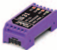
#31 PIC-based ADC and PWM
