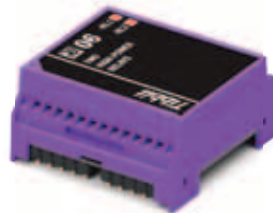
#06 Two high-power relays
