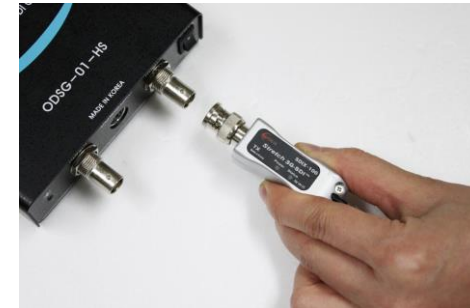
Figure 2 – Tx module of SDIX-100
