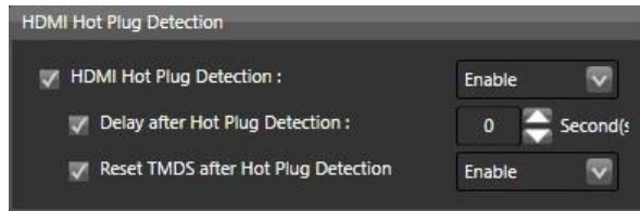
Figure. 31-4 Encoder Device Setup – HDMI Hot Plug Detection
