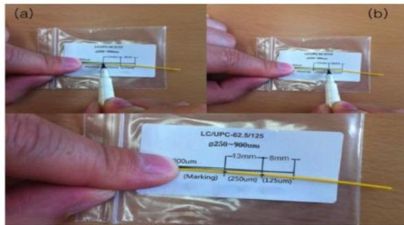
2). Mark on the tight buffer (900um) with (a), (b) for strip
